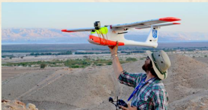
Researcher Austin “Chad” Hill prepares to launch a Skywalker 1680 FPV drone with an attached GoPro Hero camera and a Canon S100 digital camera at the site of Fifa, Jordan. The drone was also running an APM 2.6 flight control computer. ■ MORAG KERSEL
